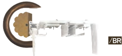
DOUBLE TRACK SYSTEM with "C" Rings, Cord Draw, Pinch Pleat, Reeded or Smooth, 2" or 3" D, 2 ½" - 4 ½" rear return, 5 ½" - 7" front return *Fascia not available on the back track
