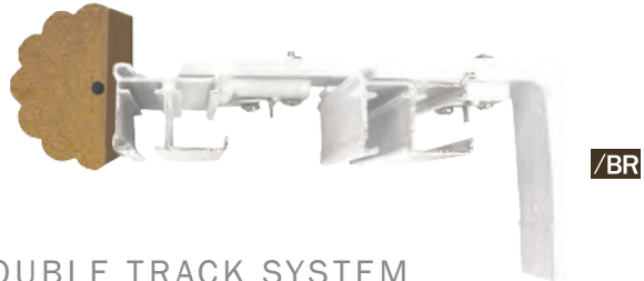
DOUBLE TRACK SYSTEM Cord Draw, Ripplefold or Pinch Pleat, Reeded or Smooth, 2" or 3" D, 2 ½" - 4 ½" rear return, 5 ½" - 7" front return *Fascia not available on the back track
